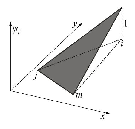
$\psi$  is called the *shape function*. Elements with a linear shape function are called linear elements, and  $\psi_i$  is typically as on the figure, i.e.  $\psi_i$  is 1 in node i, and 0 in the other nodes.
