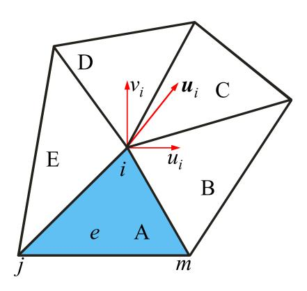
Figure shows part of our mesh, with some elements surrounding node *i*. (On figure elements A, B, C, D, E.) Think triangles, but "any" shapes allowed. General element is called *e*, with nodes *i*, *j*, and *m*.
