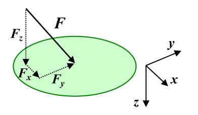
Perpendicular: Normal stress:  $\sigma = F_z / A$
