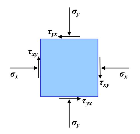
Figure shows *xy*-view of stresses acting on an elementary volume *dV*
