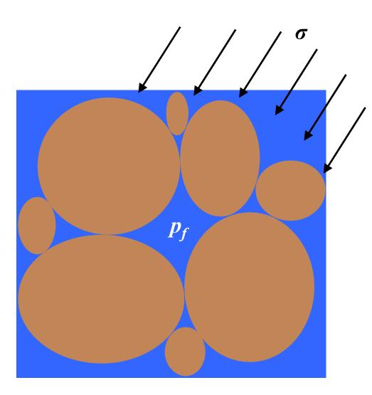
In a porous rock, the main mechanism is deformation of the pore space, not the solid itself. The force acting on the pore walls is the external stress  $\sigma$  and an opposing force by the fluid pressure  $p_{f}$ .
