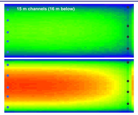
Correct modelling: (compaction computed from strain by stress simulator)
