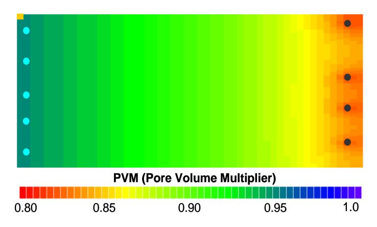
Compaction (by Pore Volume Multiplier) in Tarbert 2, in a West-East water drive.
