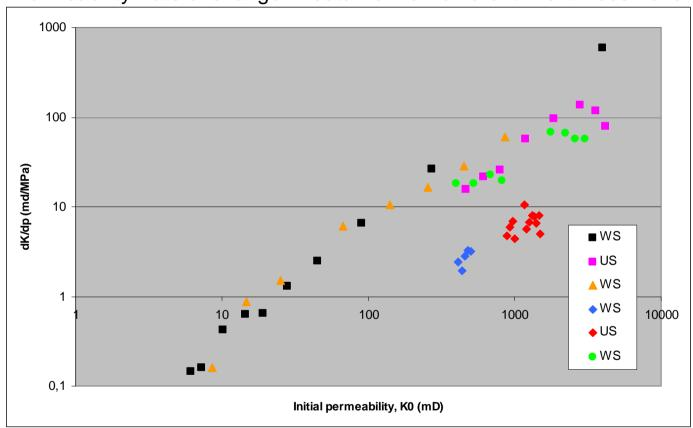
Grain pack model: Rock under compression becomes increasingly harder to compress.
