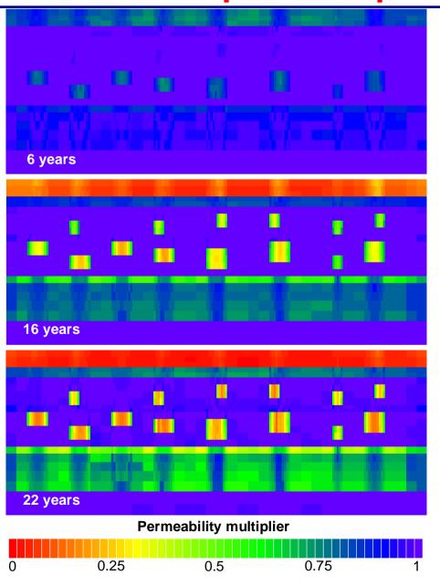
Permeability multiplier in a (YZ) cross-section transverse to channels, near Upper Brent producers.
