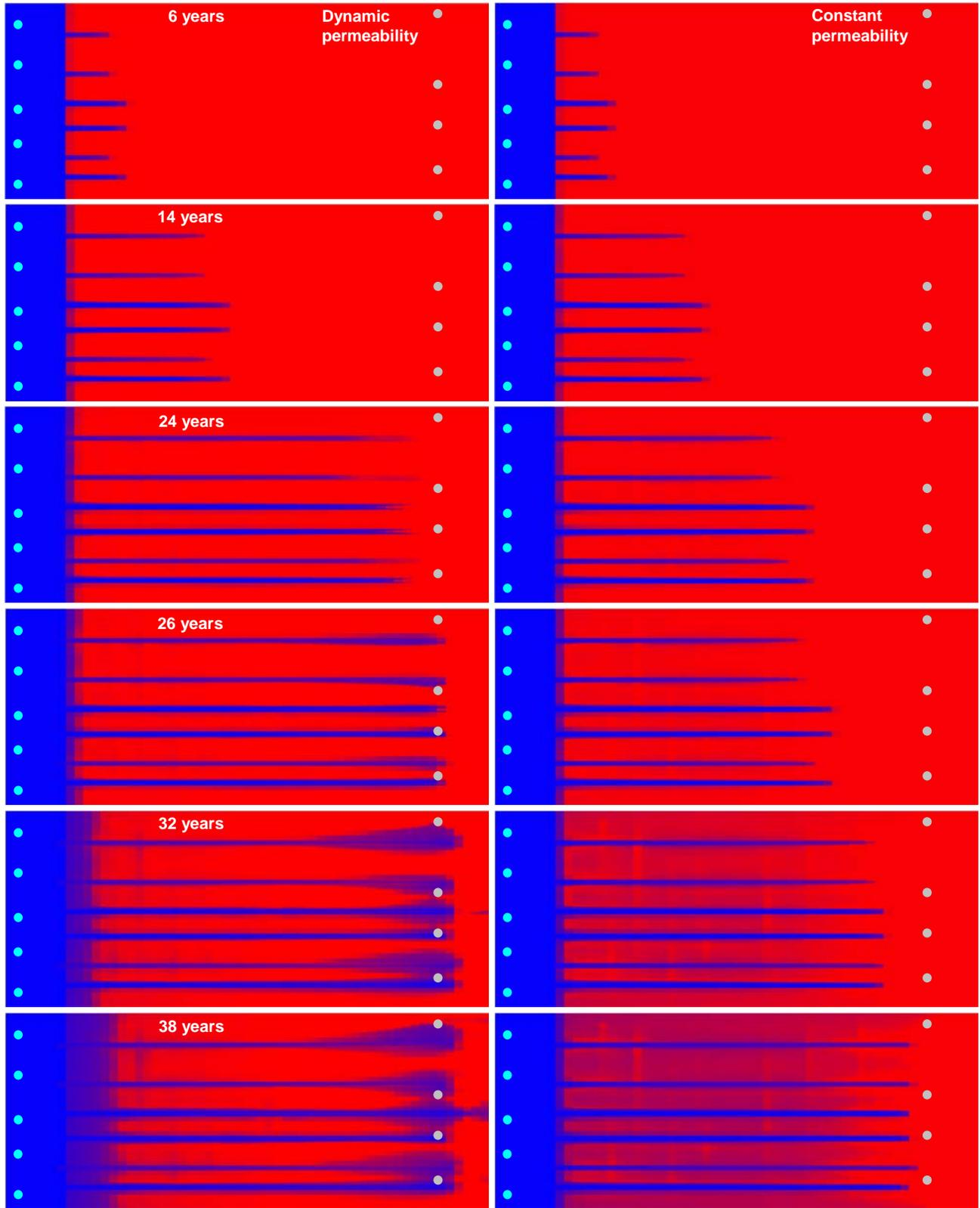
**Fig. (12).** Water saturation in a Ness 2 grid layer containing 50 m wide channels, LC case. Water injectors to left (West), Upper Brent oil producers to right (East) (light gray). Blue is water, red oil.
